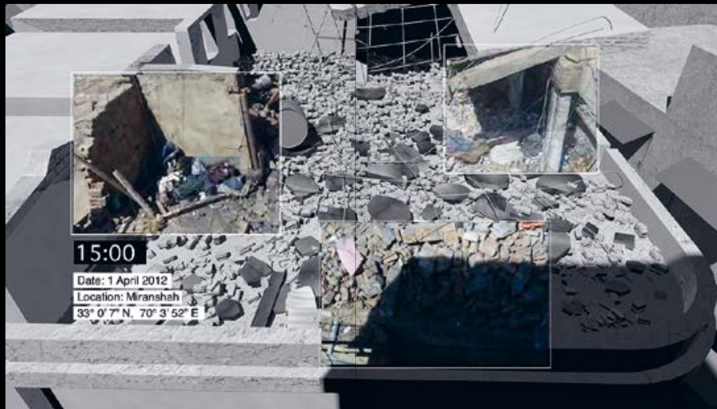
Drone Strike in Miranshah (2016) . A composite image merges news footage of a home destroyed in a drone strike on Miranshah, North Waziristan, Pakistan, together with Forensic Architecture's 3-D modelling. Forensic Architecture used shadow analysis to corroborate the approximate time (15:00) the video was shot. Courtesy of Forensic Architecture.
